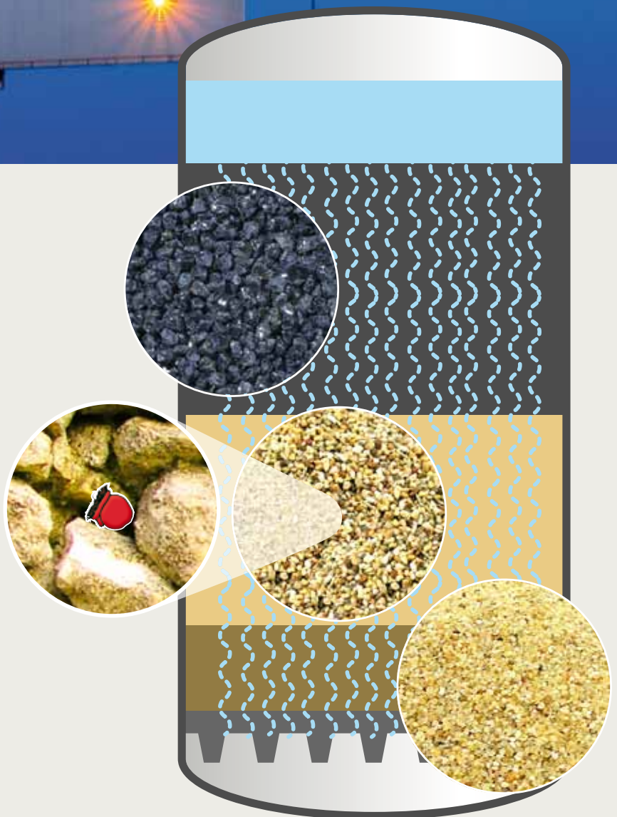
Fig. 21 Gravel filter construction
